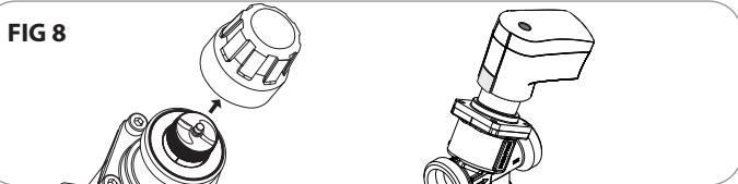
**EN FIG 8: Mount the actuator on the valve.**
