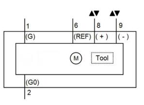
Note: The operating voltage at terminals G and G0 must comply with the requirements under SELV or PELV. Safety transformers with twofold insulation as per EN 61558 required; they must be designed to be on 100 % of the time.
