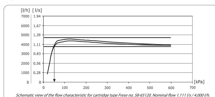
The cartridge enters the pressure range at 47 kPa and maintains the flow at a constant level to 600 kPa.
