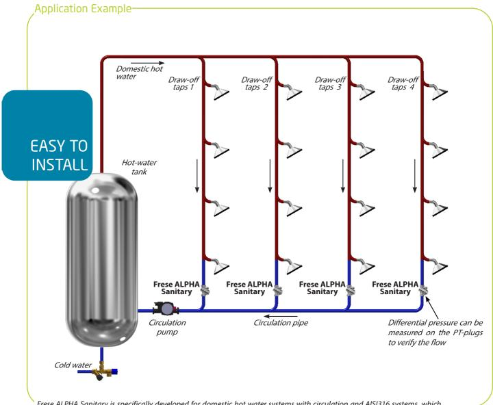
Frese ALPHA Sanitary is specifically developed for domestic hot water systems with circulation and AlSI316 systems, which require high corrosion resistance.
