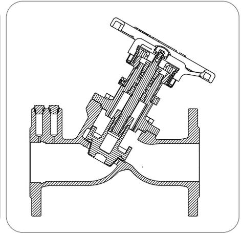
*DN350-DN500 section drawing*
