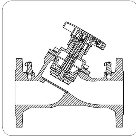
*DN65-DN300 section drawing*
