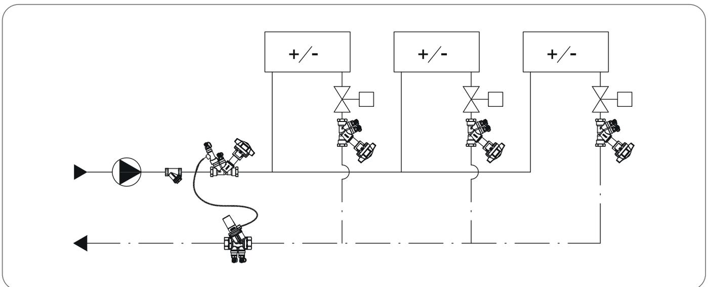
The STBV VODRV valve is placed on every coil to verify and balance the flow.
