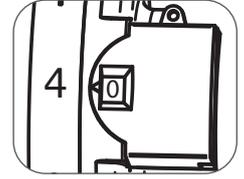
Frese STBV VODRV is set using the pre-setting scale located below the handwheel. The set point of the valve can be determined by using the tables from page 9.
