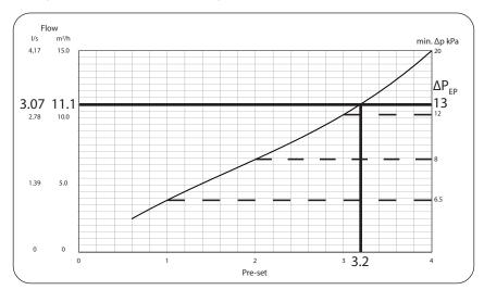
The selected OPTIMA Compact EP DN50 LF requires  $\Delta P_{EP} = 13$  kPa of differential pressure and should be set to position 3.2 to provide the sizing flow.
