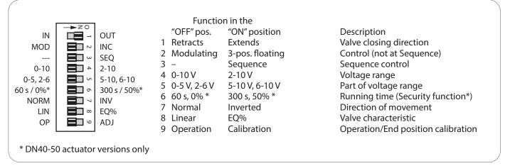
There are nine switches in a row on the circuit board. On delivery ('Factory'), all switches are pre-set as above.
