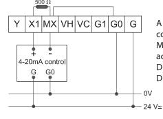
A 500  $\Omega$  resistor must be connected between X1 and MX. (Not delivered with the actuator)
