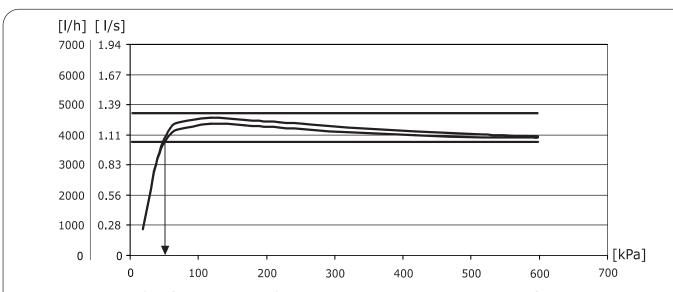
Schematic view of the flow characteristic for cartridge type Frese no. 58-65120. Nominal flow 1.111 l/s / 4,000 l/h. The cartridge enters the pressure range at 47 kPa and maintains the flow at a constant level to 600 kPa.
