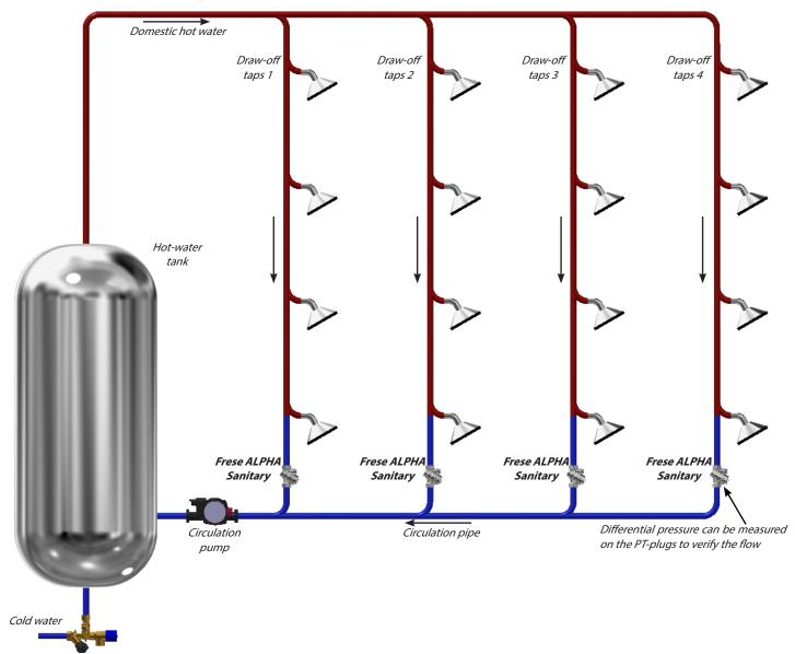
Frese makes three different valves for domestic hot water circulation: Frese CirCon, Frese TemCon and Frese ALPHA Sanitary.
