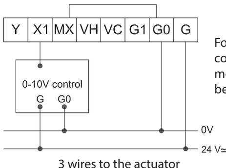
For 0-10V control with 3 wire connection, it is needed to mount an internal wiring between MX and G0
