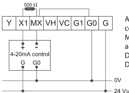
A 500 Ω resistor must be connected between X1 and MX. (Not delivered with the actuator)
