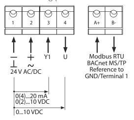
Electric wiring (With cable - 48-5394)
