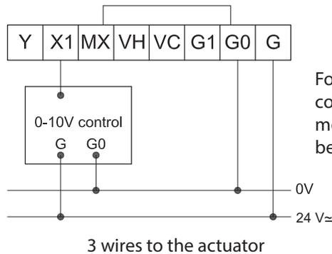
For 0-10V control with 3 wire connection, it is needed to mount an internal wiring between MX and G0
